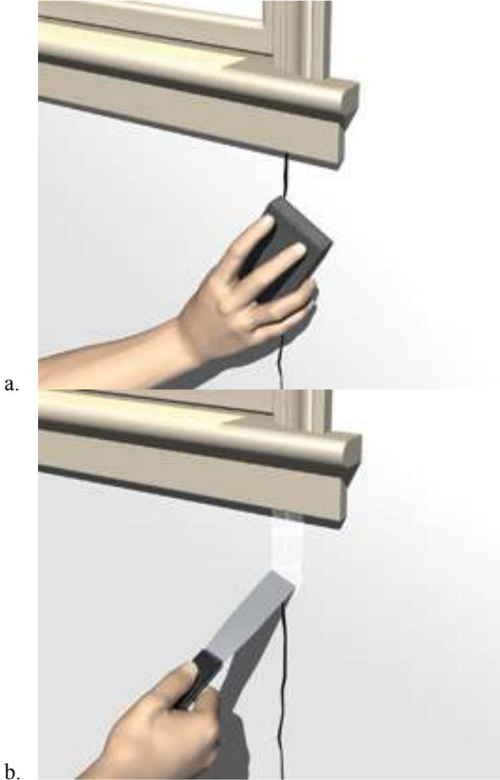
3. To correct a nail / screw pop, reset the nail with a hammer and punch/ screw driver. See illustrations below.
